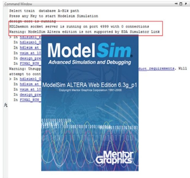
Figure 5: HDLDAEMON as the interface between MATLAB and ALTERA-Model Sim
