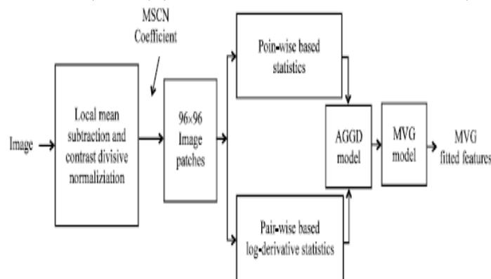
Figure 1: Block diagram of the proposed algorithm for features extraction. Where MSCN stands for mean subtraction and contrast divisive normalization, AGGD is asymmetric generalized gaussian distribution and MVG represents multivariate gaussian model
