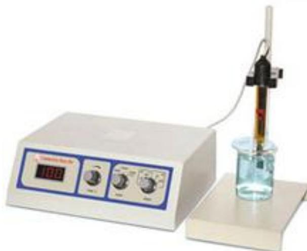
**Figure 1:** The pH-meter for acid-base titration
