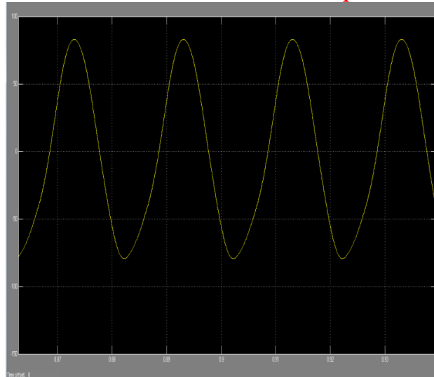
Figure 7: Simulation graph for transformer-less full bridge inverter Voltage ripple for transformer-less full bridge inverter is 65% and efficiency produced is 75%.
