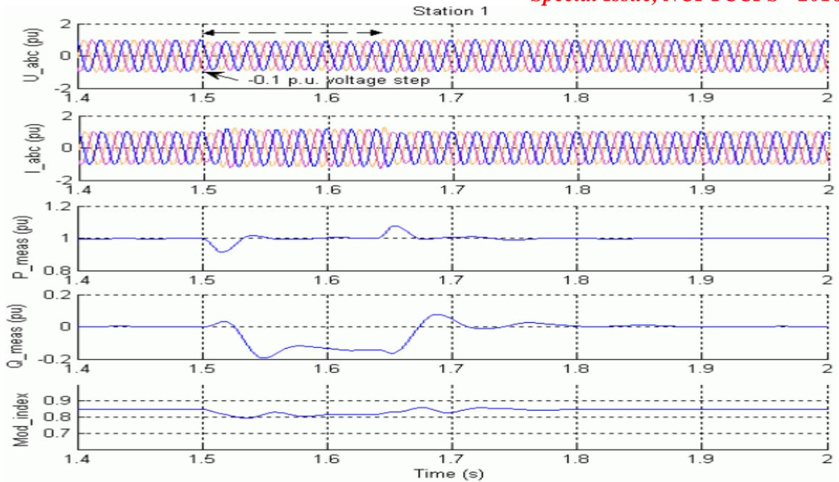
Figure 5: Voltage Step on AC System 1
