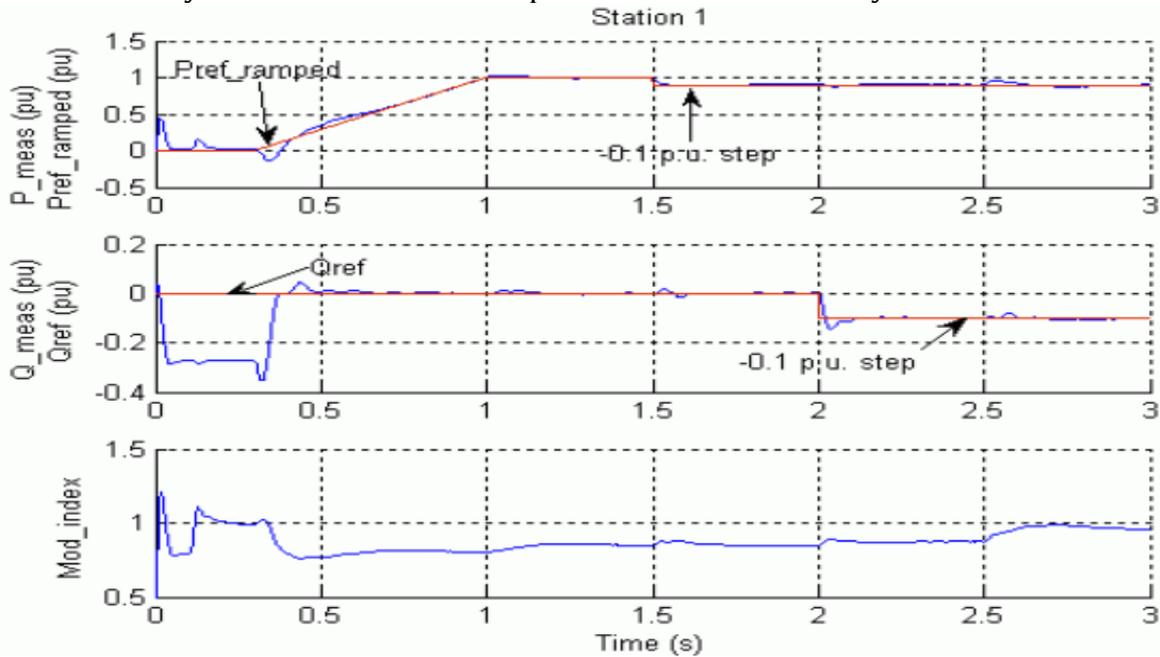
Figure 3: Startup and P & Q Step Responses in Station 1
