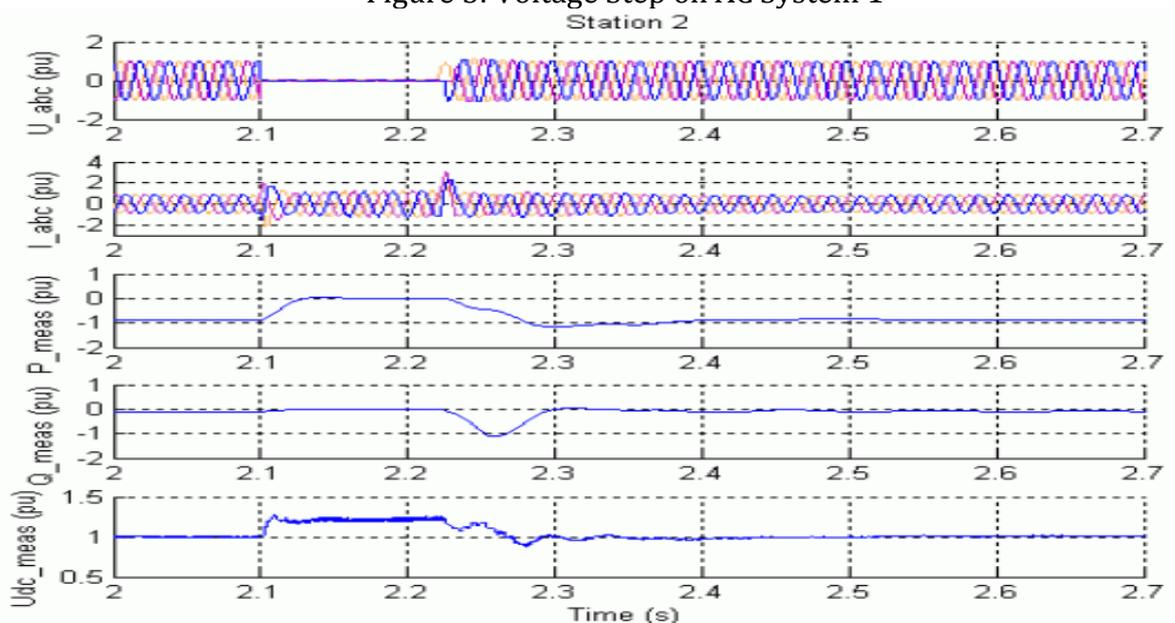
Figure 6: Three Phase to Ground Fault at Station 2 Bus
