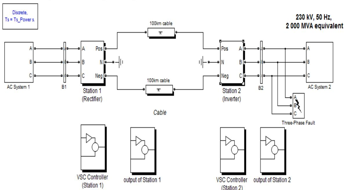
Figure 2: VSC-HVDC Transmission System Model
