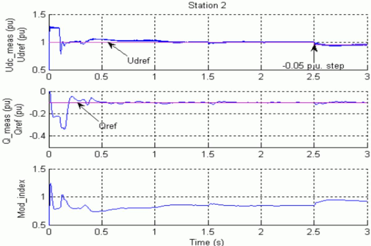
Figure 4: Startup and Udc Step Response in Station 2
