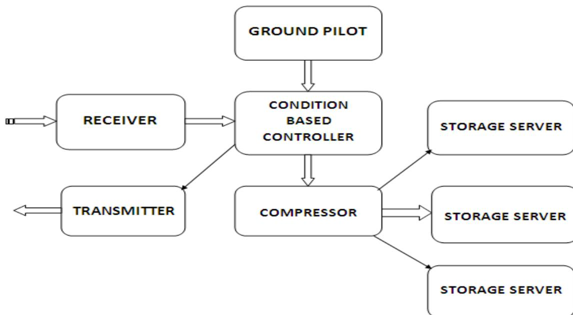
**Figure 1.5: Block diagram for overview of Ground station**
