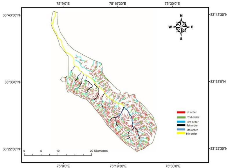
Figure 3: Showing Drainage map of Sandran stream
