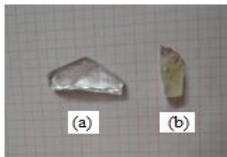
Figure 1: The grown crystals of (a) undoped and (b) ferric sulfate doped KDP crystals
